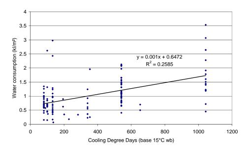
Figure 4. Water consumption versus cooling degree days.
